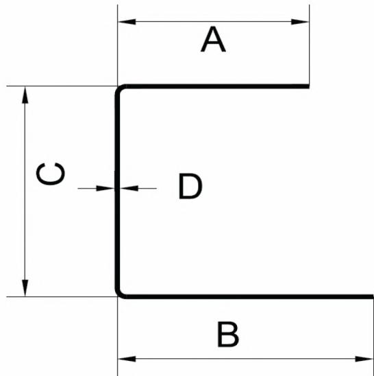
**False Ceiling GM 50 Perimeter Channel framing:**
